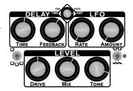
Lead Fattener: Make your solo stand out of the mix. Bonus points if you turn your amp to 11. (Modulation off) Alternatively, try a hair of modulation with RATE around 12:00 and just a hair on the AMOUNT knob
