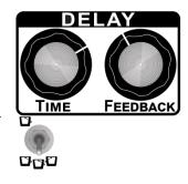
Note: as delay times lengthens high frequency roll off changes. In addition, very short or very long delay times will have reduced gain. Therefore, the tone or feedback levels may be different in 1 or 3 bucket mode or the standard ADG-1 in 2 bucket mode, even if the delay time is the same.
